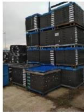
Dunnage trays made of recycled EPP
