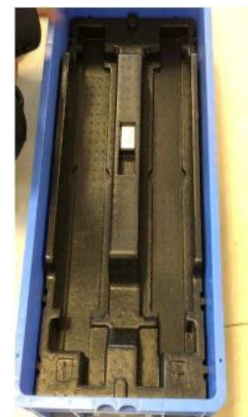
An expanded polypropylene (EPP) box inside an injection box
